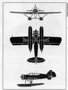
Most Japanese I-15 class subs carried a Glen (Type Zero E14Y1) floatplane designed at Yokosuka Navy Arsenal and built by Kyushu. Craft was started inside deck hangar, then rolled out and its wings unfolded; launched by catapult, retrieved at mission's end with crane. Such a plane from the I-25 twice bombed southern Oregon.
